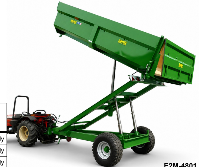
E2M-4801 with Hydraulic door control system
