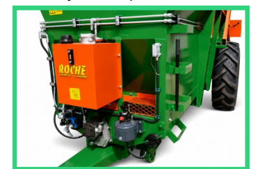
Hydraulic power unit
